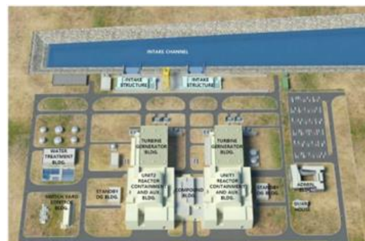
Plant Layout Arrangement
